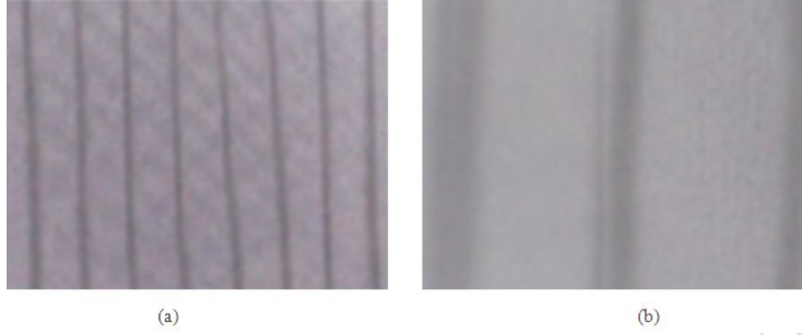
Fig. 5. Examples of moiré patterns in printed samples. The aspect ratio is 0.33 in (a) and 0.58 in (b); the ratio of periods is 0.72 and 0.44, resp. Reproduced with permission from [21]. © The Optical Society.
